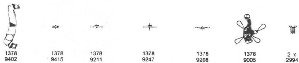
Owing to the magnetic force existing between the magnet and the stator, the rotor (1378.9415) remains suspended between its two bearings.
